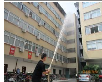
Photo of fire safety equipment Fire hydrant tested.JPG
