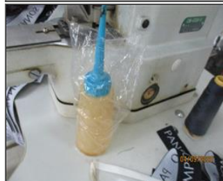
Photo of non-conformity 7.7. No safety label.JPG
